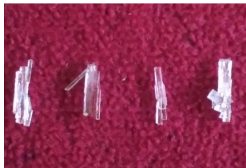
Fig. 1 Photograph of as grown LTMA single crystal
